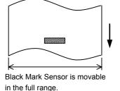
*NOTE:* Be careful the Media Guides do not squeeze the media. Doing so bends the media, causing a paper jam or feed failure. **6.** Adjust the media sensor position and select a sensor type to be used. (Refer to Section 2.9.1)
